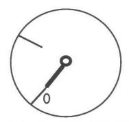
A low PSI reading (0 - 8) on the thermostat is a call for cooling.
