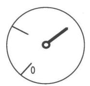
A high PSI reading (10 - ) on the thermostat is a call for heating.
